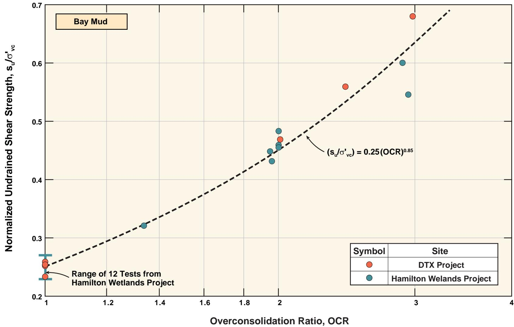
FIG\_24: Variation of Normalized Strength Ratios with Overconsolidation Ratio
