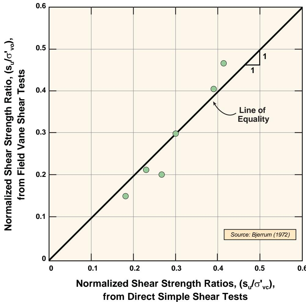
**FIG\_31:** Correlation of Normalized Strength Ratios from DSS and Vane Shear Tests
