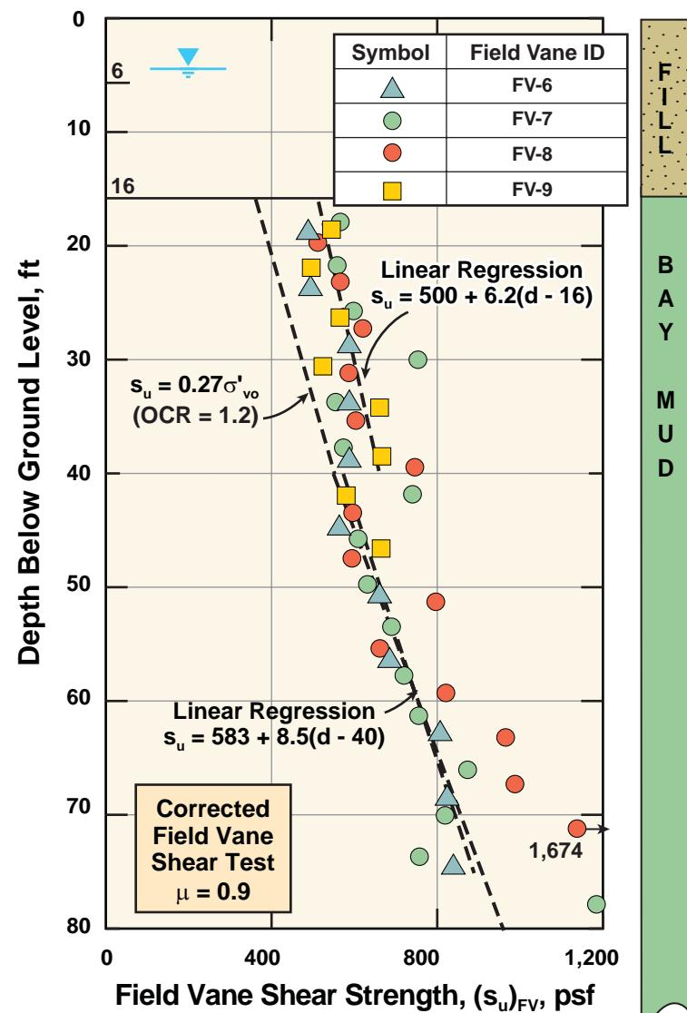
**FIG\_37: Stress History and Undrained Strengths from Vane Shear and UU Tests Islais Creek (Contract C)**
