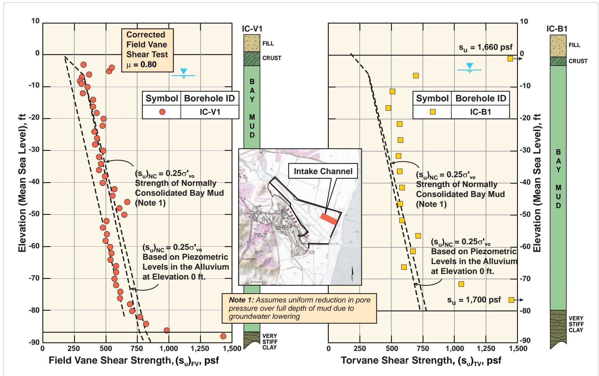
FIG\_38: Undrained Shear Strengths From Vane Shear and Torvane Tests Hamilton Field: Deep Mud Area
