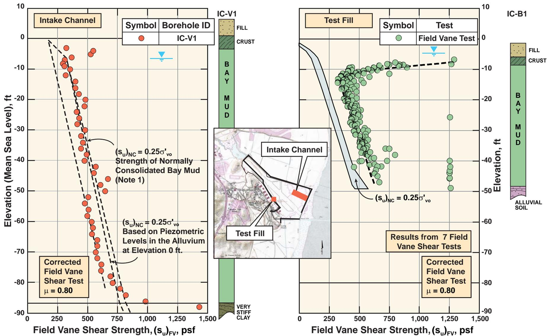
FIG\_38A: Undrained Shear Strengths From Field Vane Shear Tests Hamilton Field
