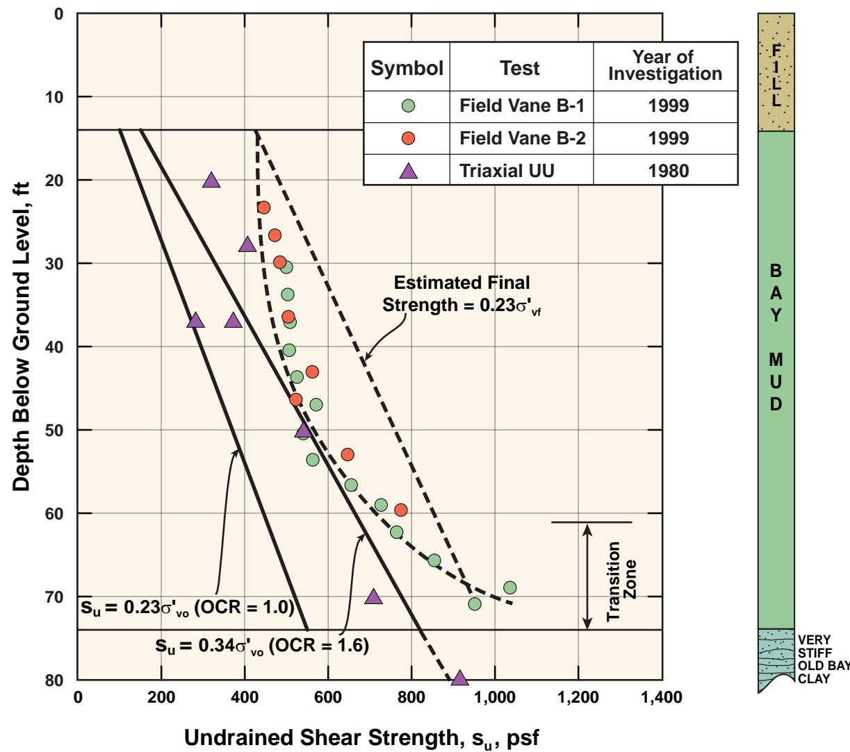
FIG\_39: Undrained Shear Strength of a Site Undergoing Consolidation Under “Recent” Reclamation Fill
