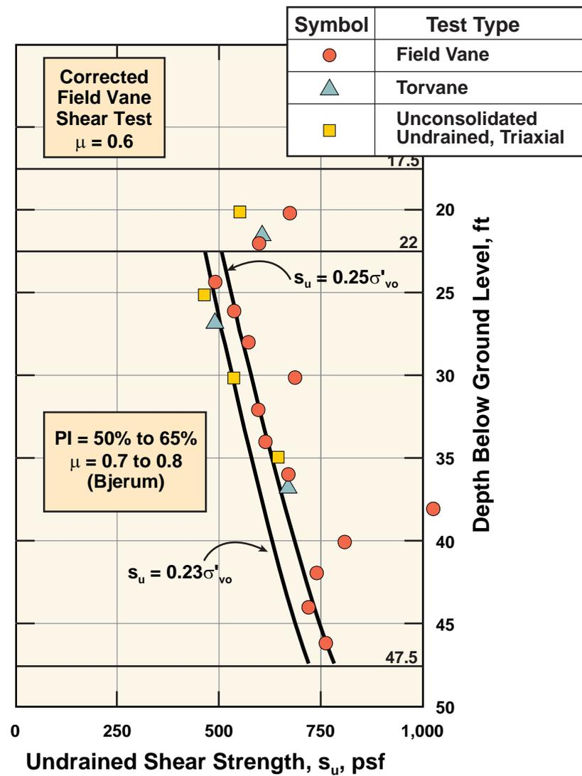
FIG\_40: Stress History and Undrained Vane Shear Strengths of Organic Bay Mud at a Recently Reclaimed Site
