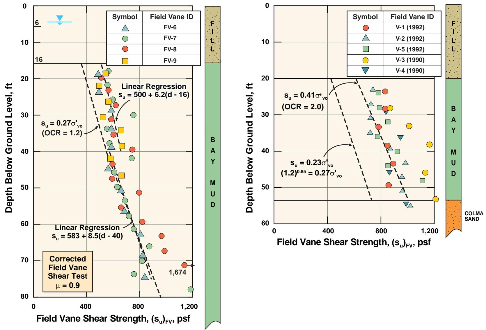
FIG\_42: Field Vane Tests Marshland Area of Islais Creek (Contract C Site)
