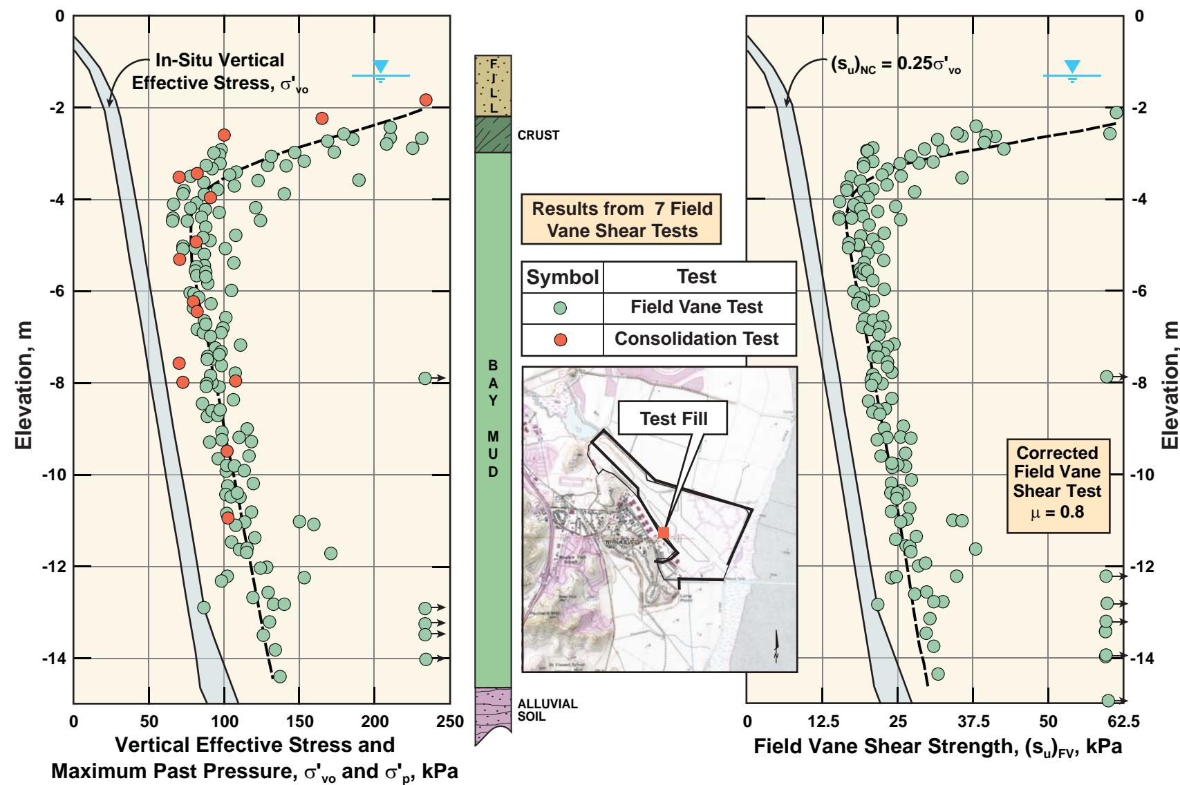
FIG\_48: Estimation of Maximum Past Pressures from Vane Shear Tests Hamilton Field Site
