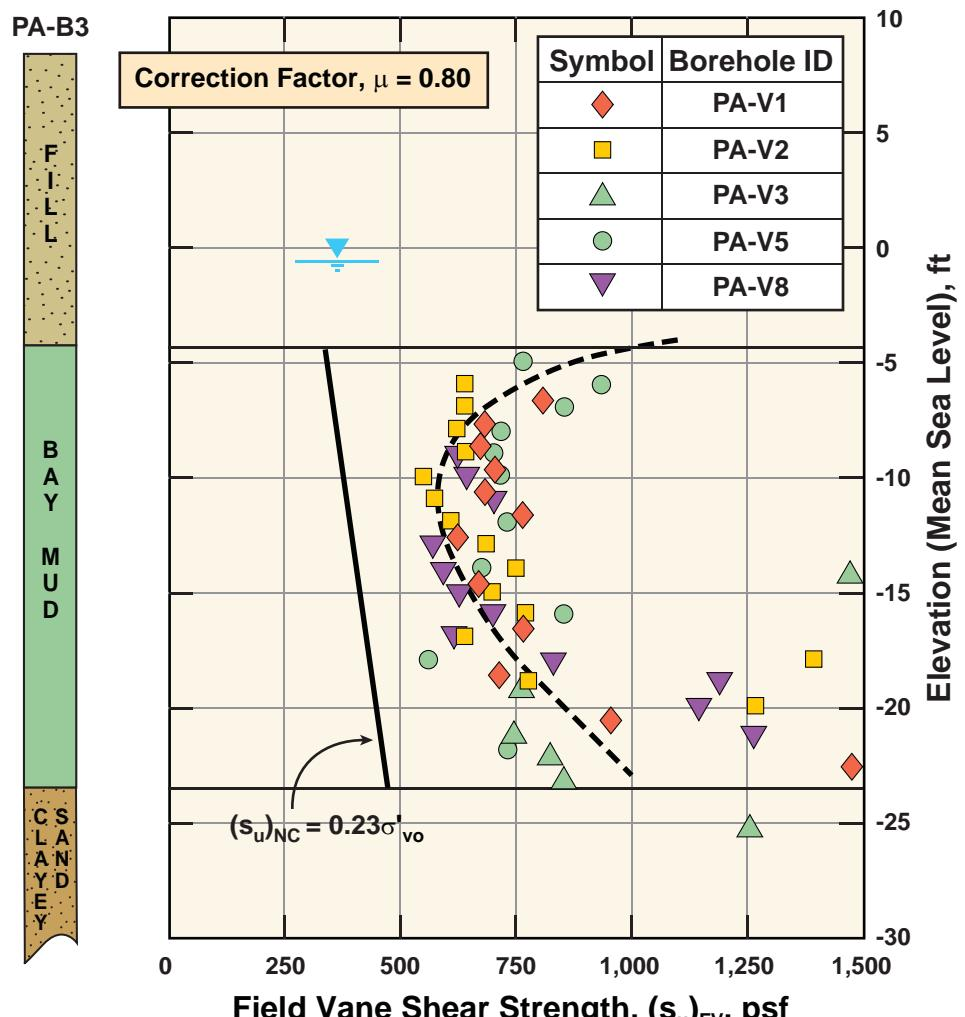
FIG\_50: Estimation of Maximum Past Pressures from Vane Shear Tests Hamilton Field Site: Shallow Mud Area Under Existing Levees
