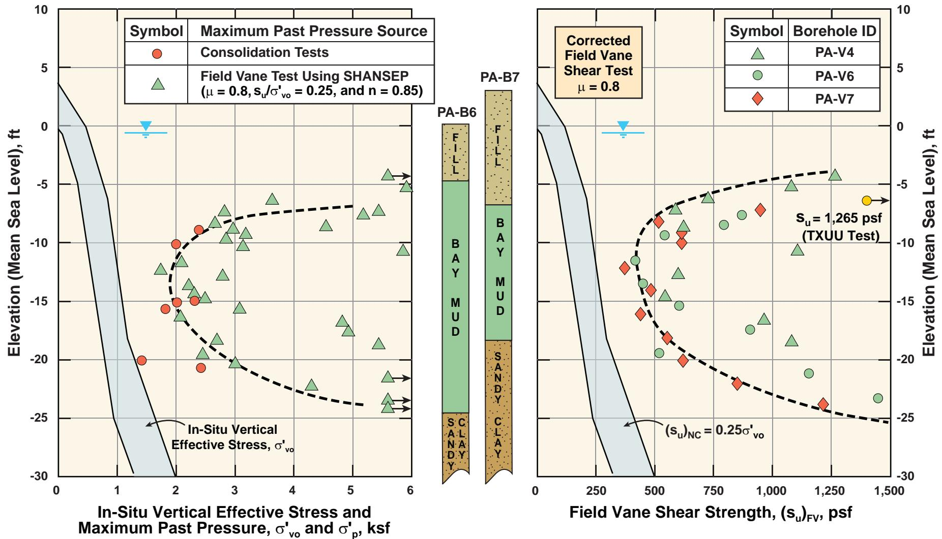
FIG\_51: Estimation of Maximum Past Pressures from Vane Shear Tests Shallow Mud – Free Field Area (HW)
