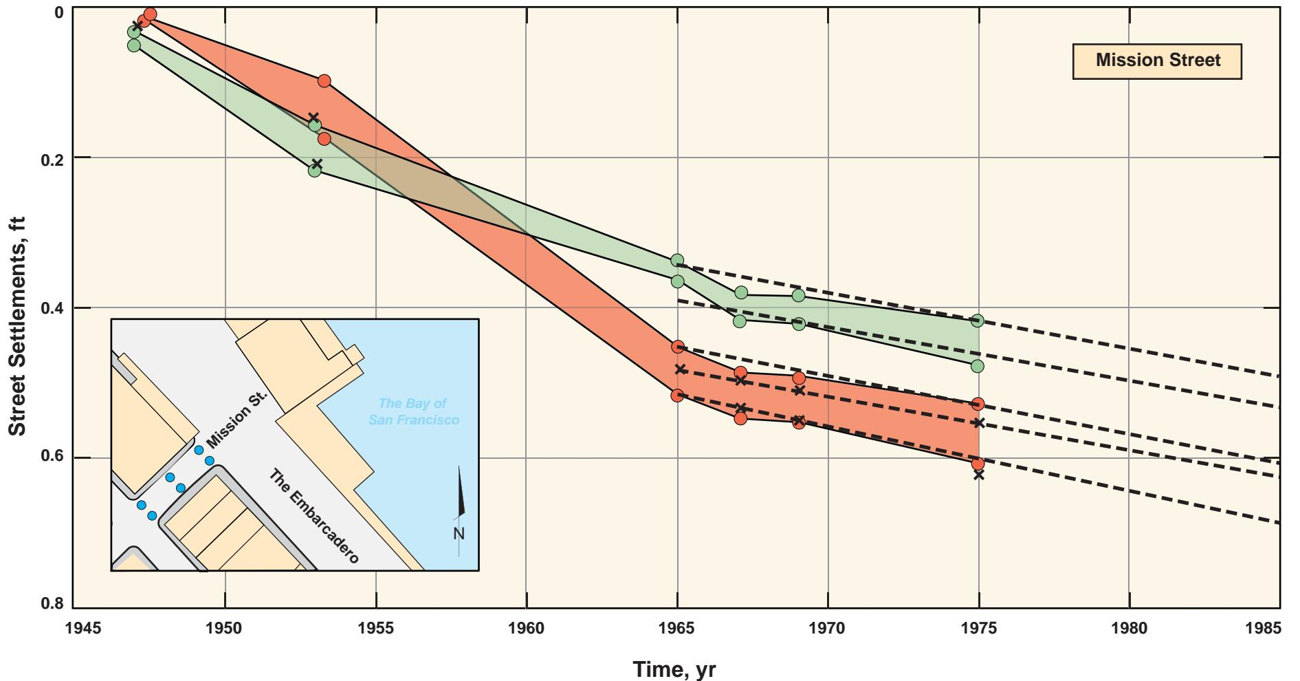
FIG\_72: Extrapolation of Settlement Data at Mission Street For Secondary Compression
