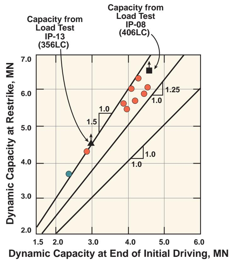
**FIG\_96:** Effects of Soil Set-Up on Driving Resistance and Axial Capacity 12 in and 16 in Concrete Piles
