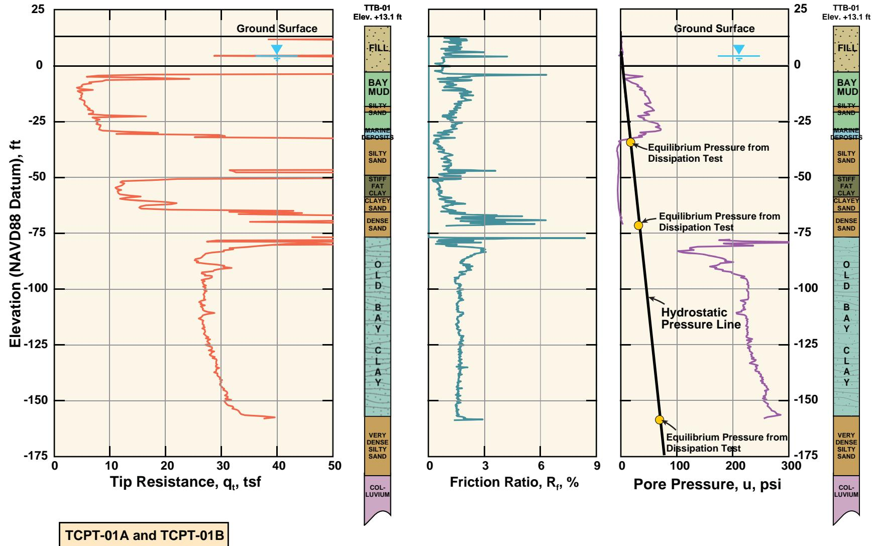
FIG\_114: Results of CPT Tests: Deep OBC East End of Transbay Terminal
