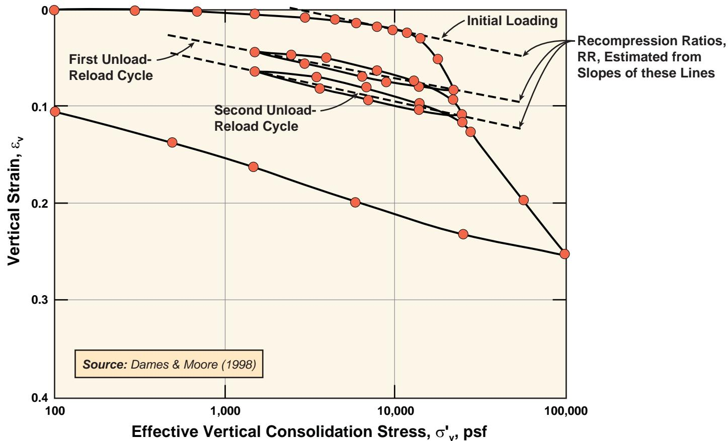
FIG\_116: Estimation of Recompression Ratio from Consolidation Tests on Old Bay Clay
