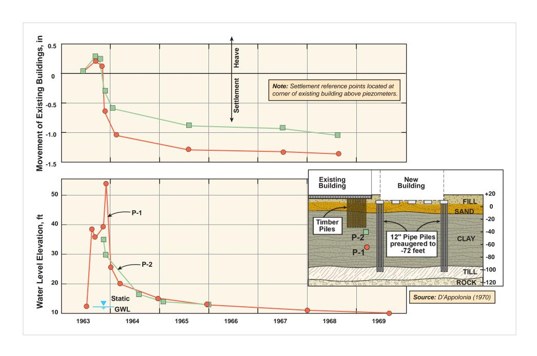
FIG\_167: Excess Pore Pressures and Movements of Nearby Building Caused by Pile Driving on the MIT Campus W:\Infrastructure\Geotech\UC Berkeley 2008 Seminar\Final Figures\08 PILES WITH FOLLOWERS\FIG\_177
