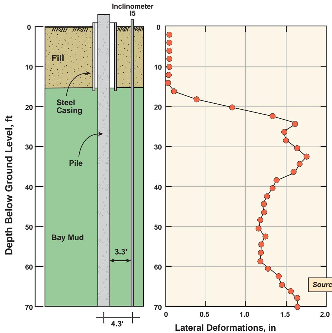
FIG\_168 : Lateral Deformations Caused By Driving A Single Pile In Bay Mud
