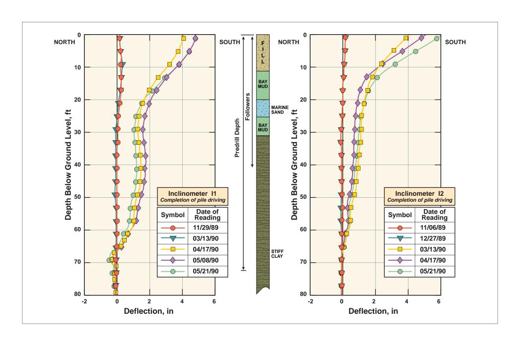
FIG\_175: Lateral Driformations Measured During Pile Driving with Deep Followers
