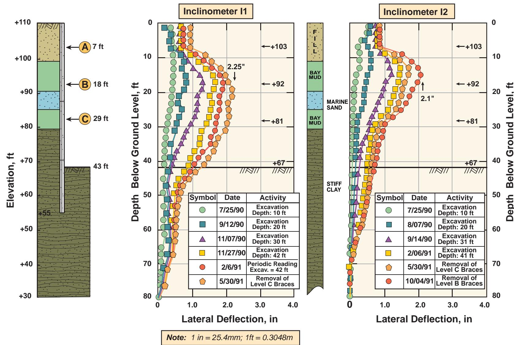
FIG\_179 : Lateral Deformation Profiles At Various Excavation Stages: Storage Basin Site
