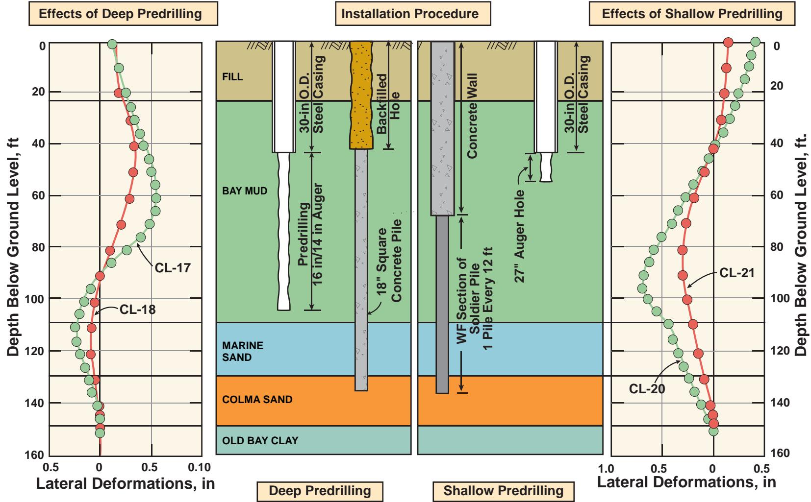
FIG\_183 : Lateral Deformations Caused By Pile Driving
