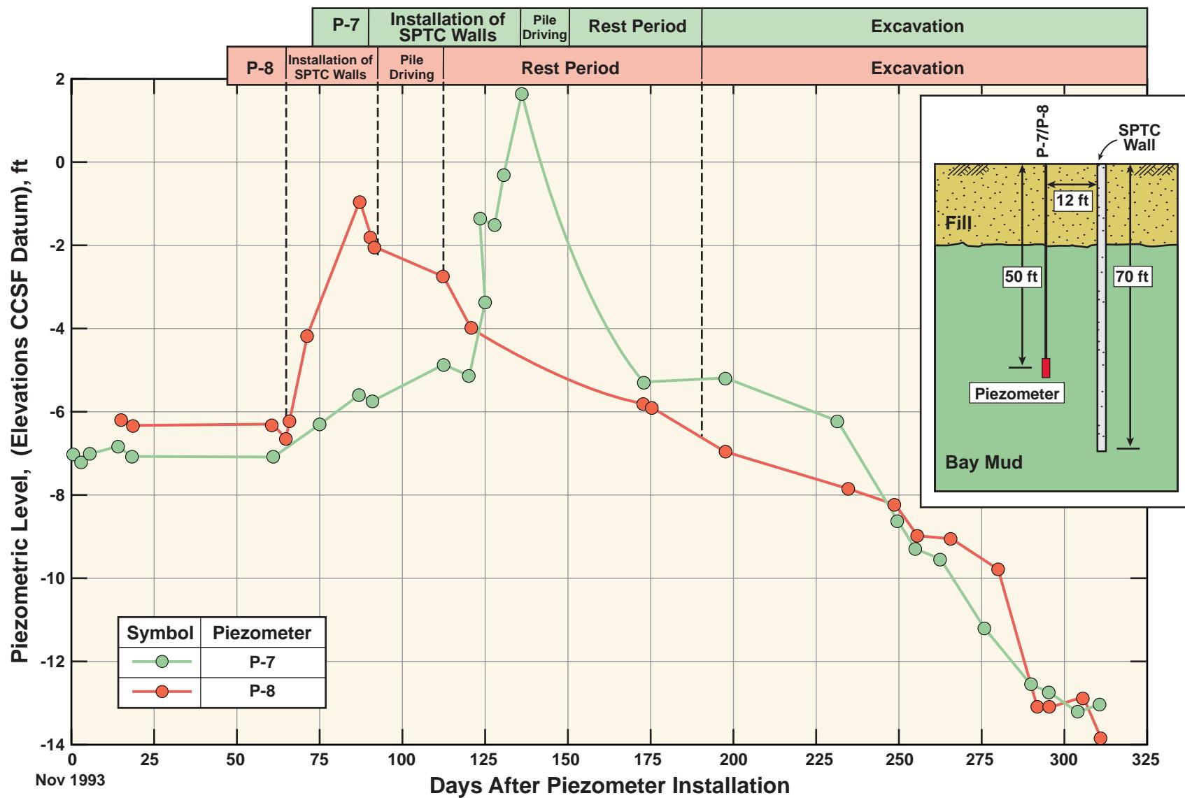
FIG\_200: Change in Pore Water Pressures: Effects of SPTC Wall Construction Pile Driving and Excavation
