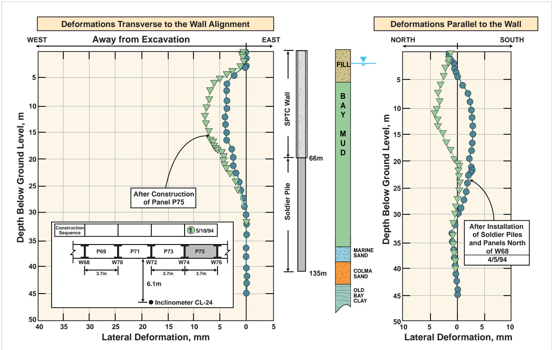
FIG\_201B: Lateral Deformations During SPTC Wall Construction
