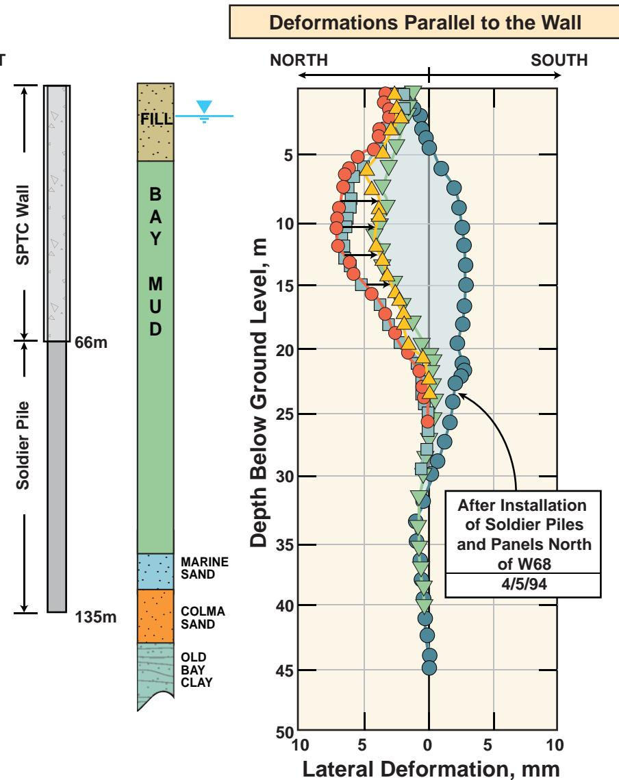
**FIG\_201E: Lateral Deformations During SPTC Wall Construction**
