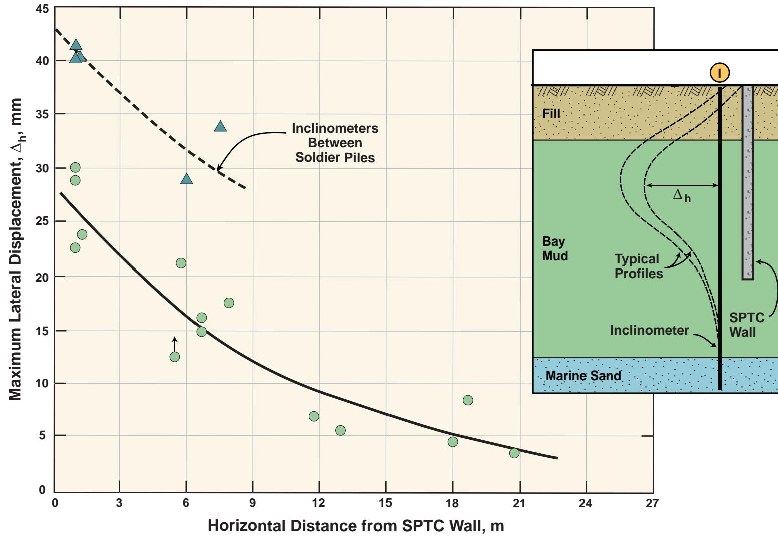
FIG\_202: Variation of Lateral Deformations with Distance from Excavation Effects of SPTC Wall Construction
