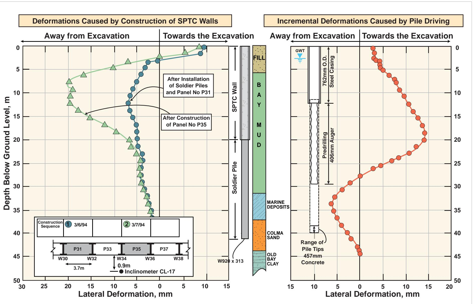
FIG\_203B: Lateral Deformations Caused by SPTC Wall Construction
