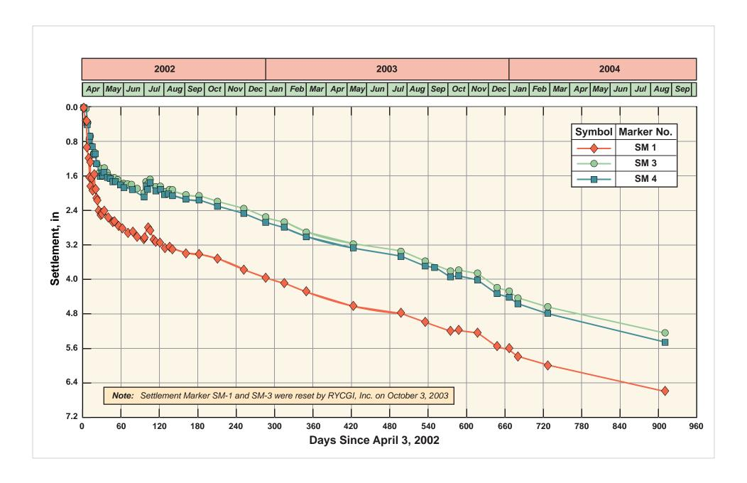
Fig\_A-07: Vertical Movements of Settlement Markers Versus Time
