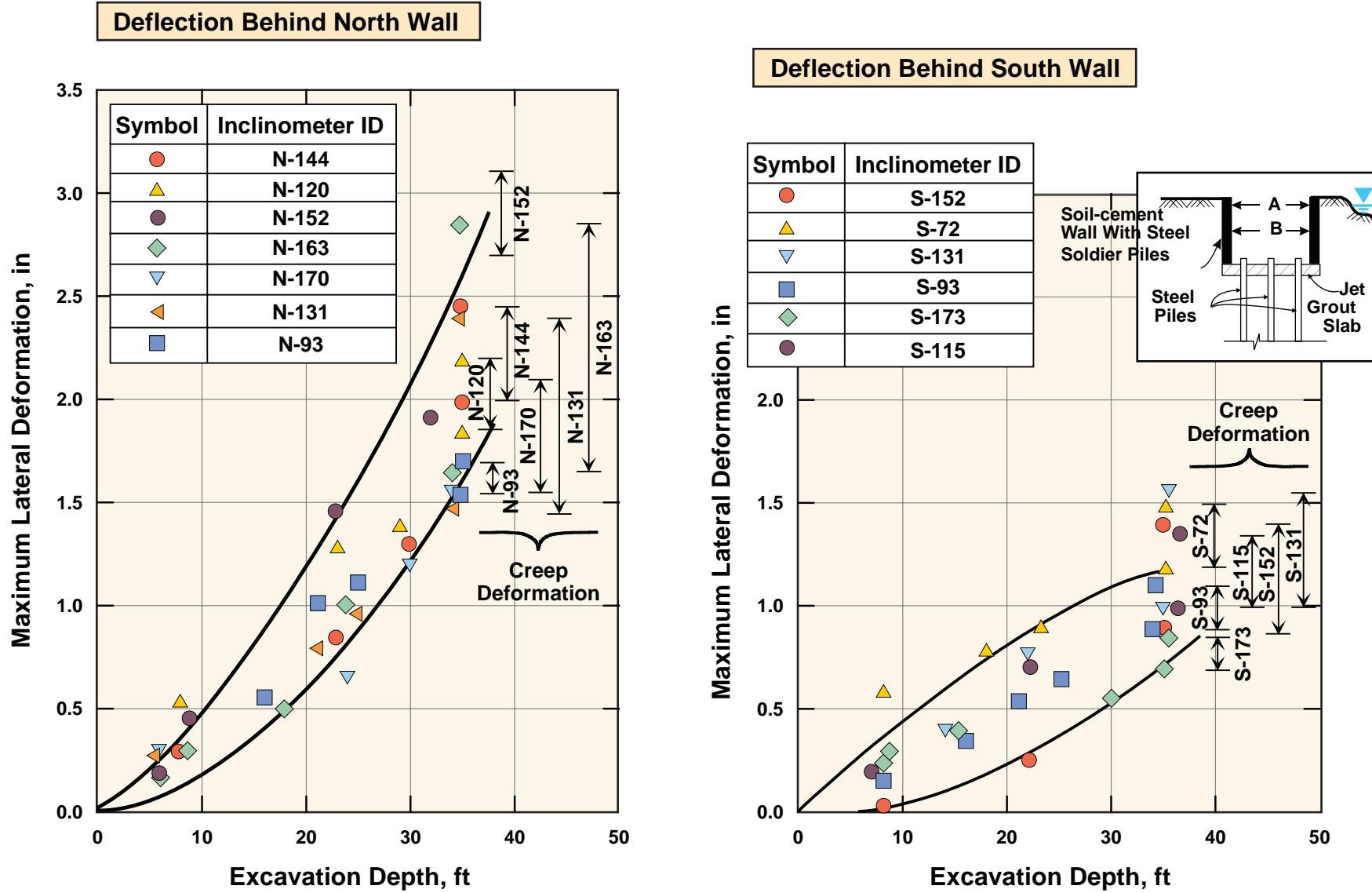
FIG\_237: Lateral Deflections Versus Excavation Depth: Overflow Structure Along Islais Creek
