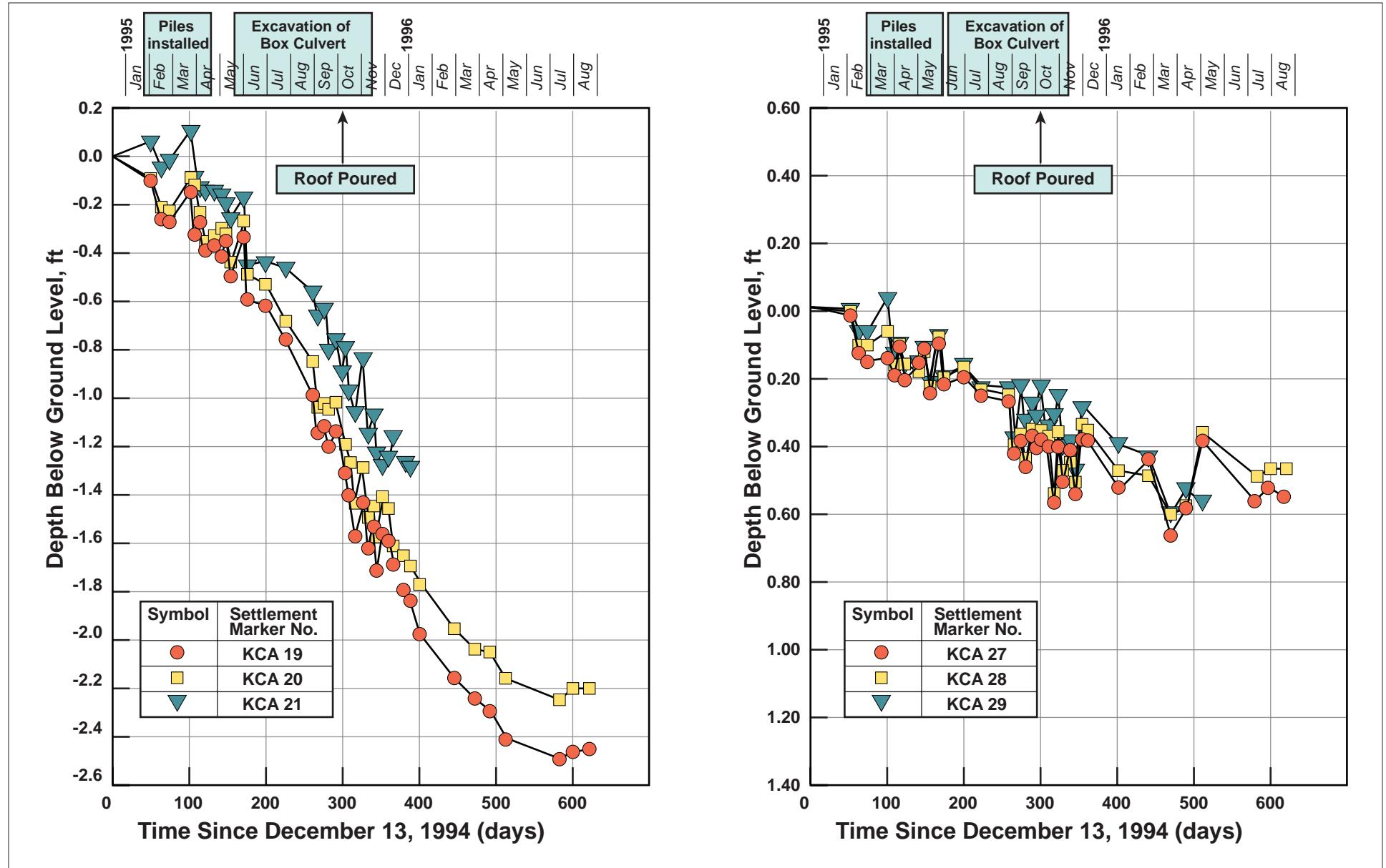
Plate D-14: Settlements Versus Time Measurement in the Area Between Marin and Army Streets
