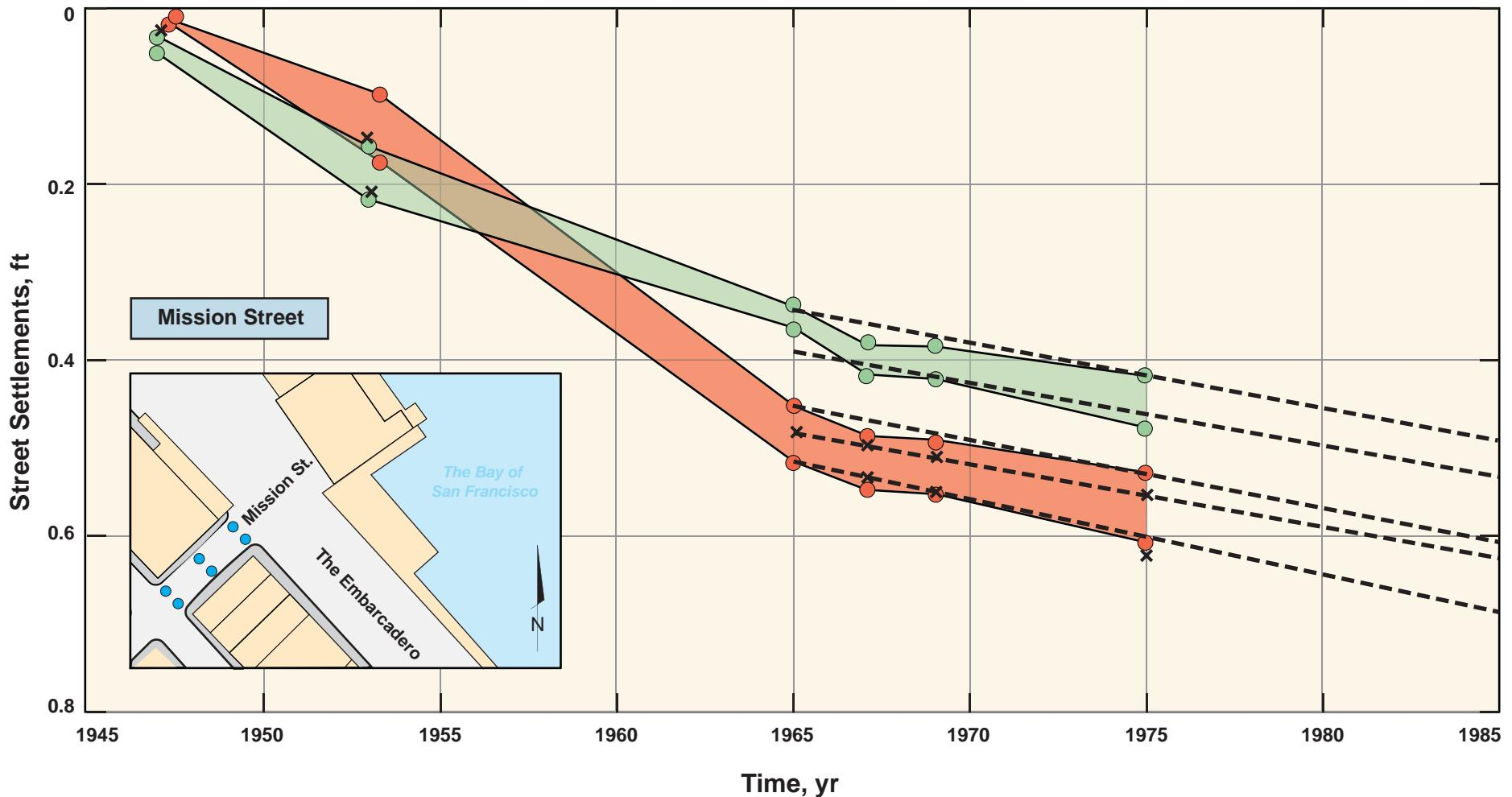
Plate E-06: Surface Settlements Measured at Howard and Mission Streets Between Steuart and Embarcadero
