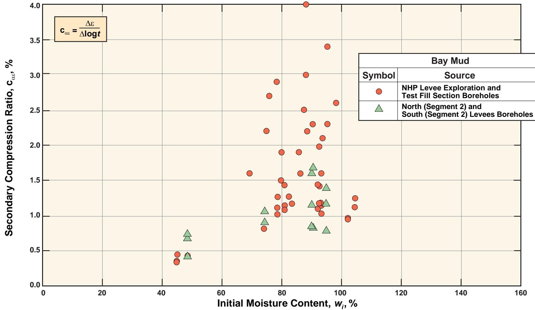
Plate P-04: Variation of Coefficient of Secondary Compression with Moisture Content
