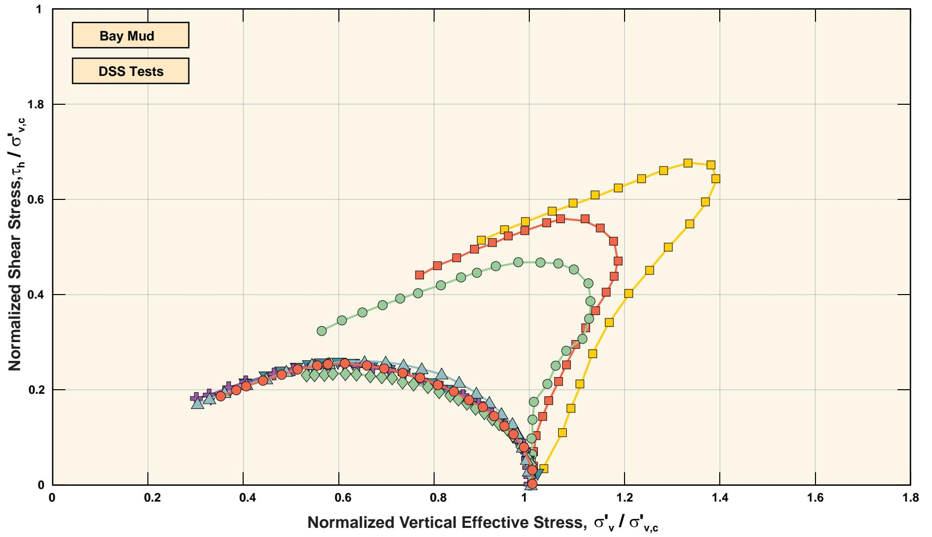
Plate GDR-62-2: Normalized Effective Stress Paths from DSS Tests on Bay Mud
