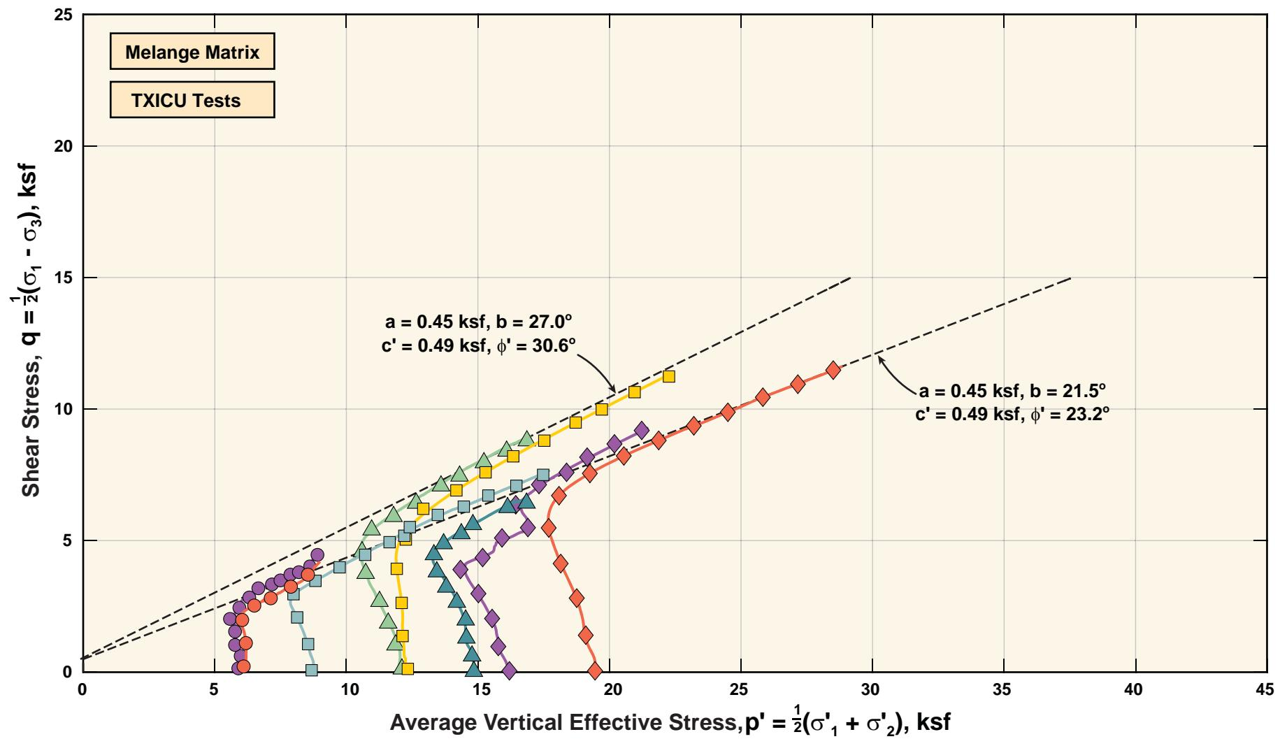
Plate GDR 79-2a: Effective Stress Paths from Triaxial Compression Tests on Melange Matrix
