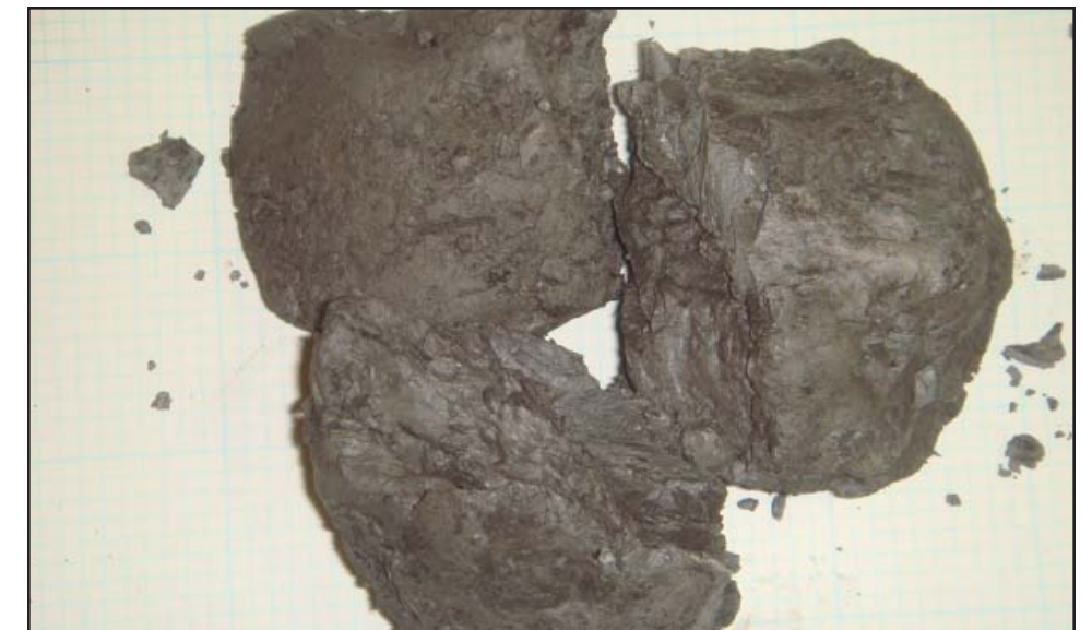
Picture 6: Close-up view that shows the presence of slickensides.
